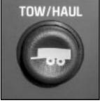
Your vehicle is equipped with a tow/haul mode. The button is located on the instrument panel to the right of the steering wheel.
